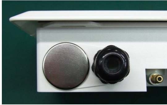
Fig. 3-8 Installed plugs on unused openings in the base.
