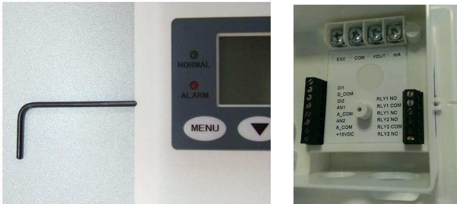
Fig. 3-3 Removing bezel from the base
